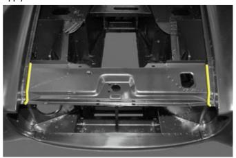
**4. Transmission tunnel and rear body**Apply to both sides of the tunnel, down into the footwell,
